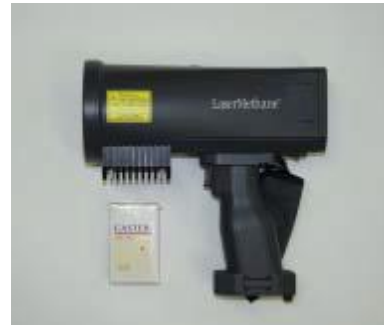
Fig. 1 A Portable Remote Laser based Methane Detector
