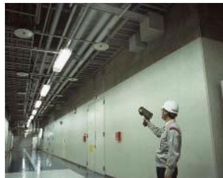
Fig. 2 An Example of How Laser based Methane Is Used
